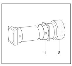
Fit the foam gasket (2) on to the connecting piece (1) on the wall pipe.
